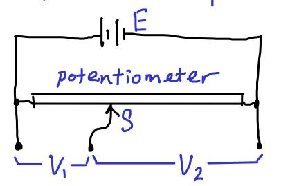
e.g. using a variable resistor like this, can adjust V, by Sliding contact S.
